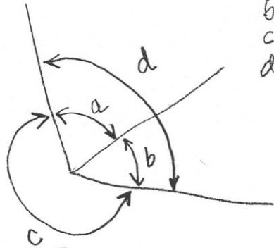
$$\begin{aligned}a &= 60^{\circ}00'00'' \\b &= 60^{\circ}00'00'' \\c &= 240^{\circ}00'25'' \\d &= 120^{\circ}00'05''\end{aligned}$$
