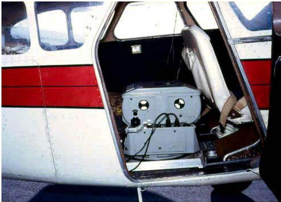
Zeiss RMK in aircraft
