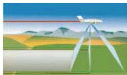
Relief of displacement in three-line-scanner imagery.
