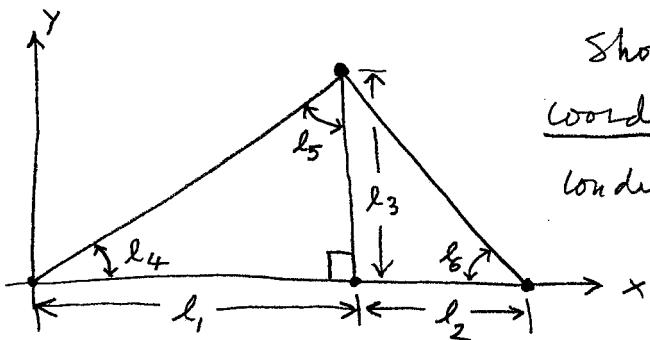
Show  $n, n_0$ , and  $r$ . Select point coordinates as parameters and write condition equations for the indirect observation method.
