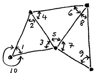
10 angles are observed to determine the shape of the figure. (a) what are  $n$ ,  $n_0$  and  $r$ ?
