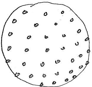
156 points observed in  $X, Y$ , and  $Z$  on the surface of a sphere:  $\sigma_x = \sigma_y = \sigma_z = 2.5 \text{ mm}$ . Estimate by LS (using mixed model)  $R, X_c, Y_c, Z_c$ . Make global test on reference variance @  $\alpha = .05$ . What are  $\sigma_{X_c}, \sigma_{Y_c}, \sigma_{Z_c}$ ?
