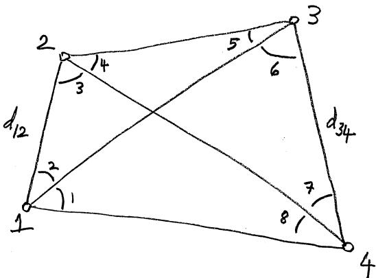
horizontal angles and horizontal distances are observed on the survey network. Estimate the station coordinates by LS (indirect obs.). Fix  $X_1, Y_1 = (100, 100)$  and  $Y_4 = 90$ . (m)
