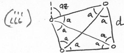
$a$  = angle observation,  $az$  = azimuth observation,  $d$  = distance observation
