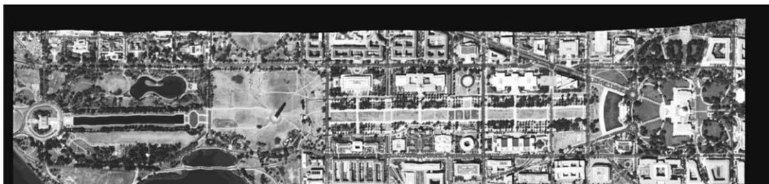
Fig. 10. Ortho-rectified image (points only, Washington, DC).
