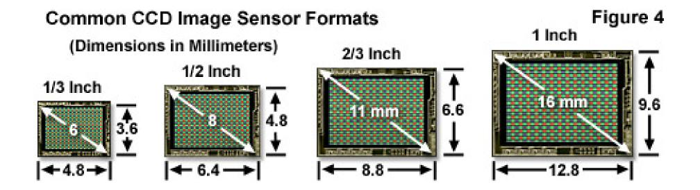
Confusing "inch" size designation of CCD arrays: diagonal is approx. 70% of active area on face of round vidicon tube with the "inch" outside diameter
