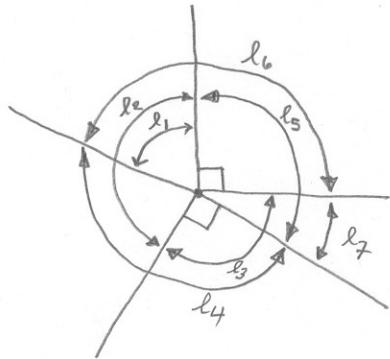
Analyze the angle figure and determine  $n$ ,  $n_0$ ,  $r$ . Note that two of the angles shown are fixed at  $90^\circ$ . Write condition equations in matrix form as
