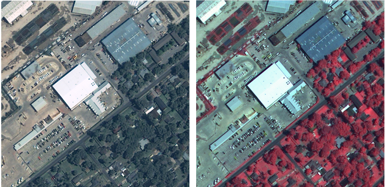
Figure 8. 4-band Pan-sharpened Product, Natural Color on the Left and Color Infrared on the Right.
