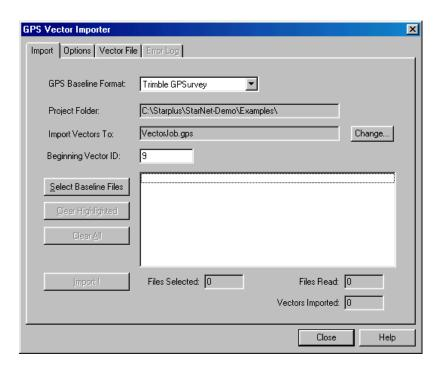
The first step in importing vectors is to choose a GPS Baseline Format from the drop down selection list. In this example we are extracting vectors from baseline files created using the Trimble GPSurvey package. Next, take a quick look at the "Options" tab. Here you can set a few options that will affect vector importing.
