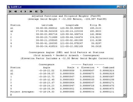
As shown above, next comes a listing of convergence angles and scale factors computed at every station in the network. The factors include the grid scale factor, the elevation factor, and the resulting combined factor.
