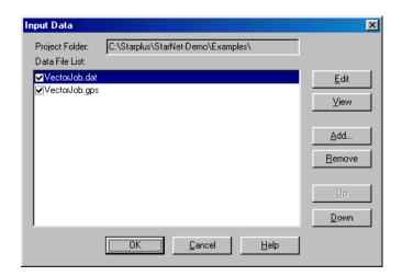
The second file contains the imported vectors for this project. For simplicity, we have <u>already</u> imported the vectors into a file for this example, and it appears in the data file list with the same name as the project, and with a "GPS" extension. In the next step, we'll actually go through the exercise of running the GPS importer to show you how this file was created.
