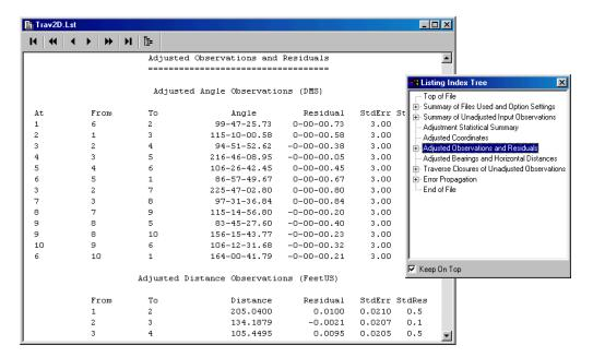
The listing file shows the results for the entire adjustment. First, locate and size the listing window large enough for your viewing convenience. This location and size will be remembered. Take a few minutes to scroll through the listing and review its contents. For quick navigation, use the tool buttons on the window frame to jump forward or backward in the file one heading at a time, a whole section at a time, or to the end or top of the file.
