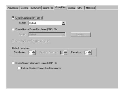
The optional "Ground Scale" file is particularly useful then running grid jobs. You can specify that the adjusted coordinates (grid coordinates in the case of a grid job) be scaled to ground surface based on a combined scale factor determined during the adjustment, or a factor given by the user. These newly-created ground coordinates can also be rotated and translated by the program.
