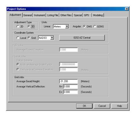
Options in the Adjustment tab are settings that describe the project. Note that the Adjustment Type is set is "3D" and the Coordinate System is set to "Grid." When a project contains GPS vectors, these two options must always be set this way. This example project is set to use NAD83 Arizona Central zone 0202.
