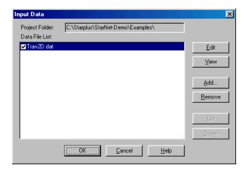
View the highlighted data file by pressing the "View" button. A view window opens so you can scroll through a file of any size. Take a minute to review the data and then close the window when finished. To edit the file rather than view it, you would press the "Edit" button, or simply double-click its name in the list.
