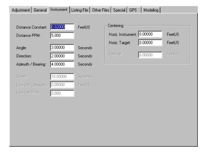
Note that instrument and target centering errors can be included to automatically inflate the standard error values for distance and angle observations. Entering horizontal centering errors causes angles with "short sights" to be less important in an adjustment than those with "long sights." Likewise, in 3D jobs, a vertical centering error can also be included to cause zenith angles with short sights to be less important in an adjustment than those with long sights.
