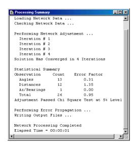
When the adjustment finishes, a short statistical summary is shown in the progress window indicating how each type of data fit the adjustment. The total error factor is shown, and an indication whether the Chi Square Test passed, a test on the "goodness" of the adjustment.
