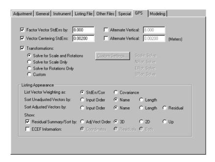
A value of 8.00 has been set for the "Factor Vector StdErrors" field which means that all the imported vector standard errors will be multiplied by this factor. Standard errors reported by many baseline processors are over-optimistic and this option allows you to make them more realistic. A "Vector Centering StdError" value of 0.002 meters has been entered which further inflates the standard errors.
