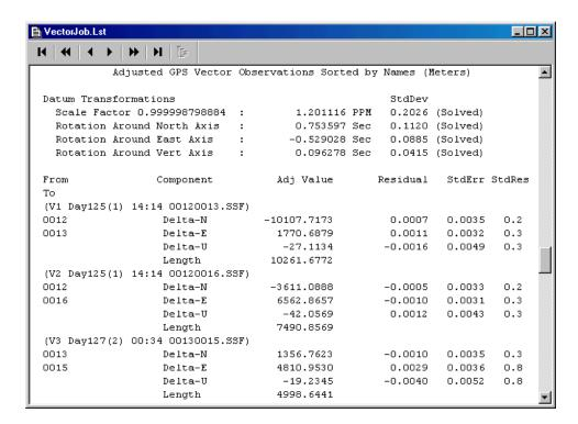
As shown above, the next output in the same section are the adjusted GPS vectors and their residuals. Always review this important section since it shows you how much STAR\*NET had to change each vector to produce a best-fit solution.
